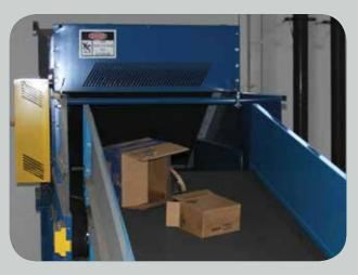
• Integrated slider bed transfer conveyor box lines available in standard and custom sizes to work in conjunction with the box crusher baler feed conveyor.
