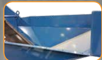
Bolt on Hopper Extensions for Versatility to Load in any Direction
