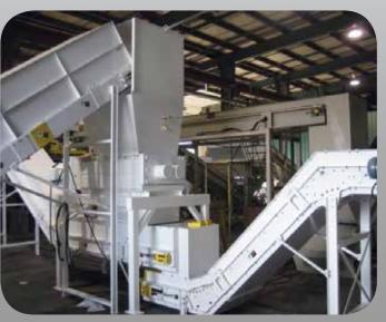
Container dumpers, infeed and discharge conveyors that are designed for any style shredding or grinding system.
