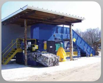
Hinged steel, combination, and slider bed belt conveyors specifically designed for feeding material into any brand of baler.
