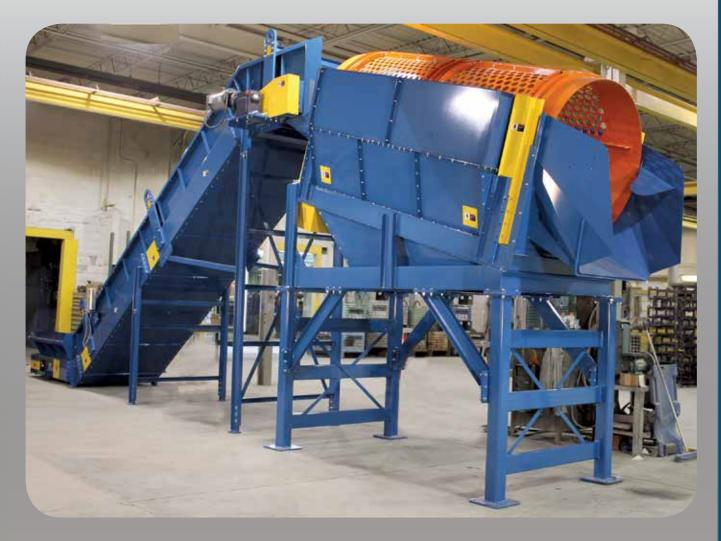
Endura-Veyor's Trommel Screens are excellent for separating different material sizes in your product stream. They can be a great addition in your sorting system for removing contaminates such as broken glass prior to hand sorting or for cleaning small debris from sorted loose materials or containers. Our designs can be built for multiple material sizes and can be changed when your screening needs change.
