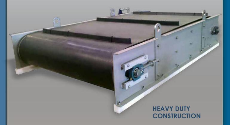
**Endura-Veyor's Overhead Magnetic Separators** are engineered and built to have a pulling range of up to 14", easily handling larger containers in current recycling markets. It will allow you to accomplish a cleaner sort by automating the process and eliminating picker error. Ferrous metal attracted by the self-cleaning model is automatically and continuously removed from the magnet face by a cleated belt.
