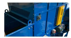
Flattening the boxes before they enter the baler allows more boxes to be handled by each baler per cycle or potentially reduce the horsepower required by each baler per cycle.
