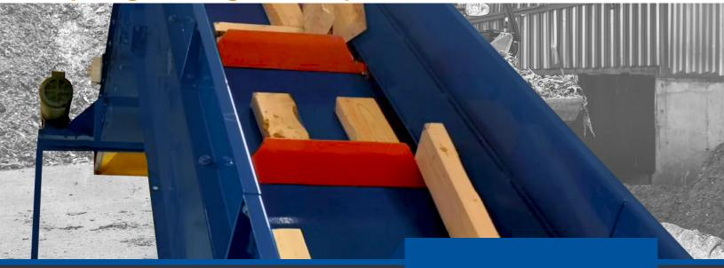
Endura-Veyor Inc.'s innovative Top Flight Drag Conveyor solves product size and jamming issues of typical drag chain conveyors. Bringing the durability of drag chain conveyors to a broader range of applications traditionally handled with Z-style fabric or steel belt conveyors.
