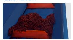
Reinforced for the environment abrasion resistant and heat resistant flights that move material along a hardened steel trough or channel.
