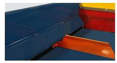
Chain driven flights provide the durability and reliability of typical drag chain conveyors and keep loose materials contained.
