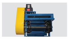
Reliable and durable, chain driven flights effectively transport and contain fine, loose materials over the long haul.
