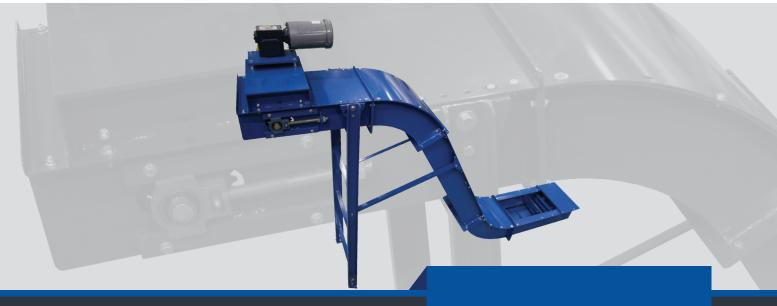
Endura-Veyor, Inc.'s Drag Chain Flight Conveyor goes beyond the capabilities of steel belt and magnetic conveyors for applications that require highly efficient handling of small, fine, abrasive, and non-ferrous materials. Flights, otherwise known as scrapers, effectively drag, collect, and transport large quantities of fine material up the incline to discharge for downstream operations.
