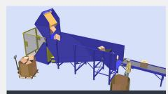
Without interrupting downstream processing, the buffering zone allows for continuous unloading of parcels while metering the flow for pre-singulation.
